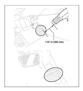
g) Heat the floor carpet area for 2 minutes as shown and smooth it out by pushing it with your hand. Heat the same area again for another minute, and smooth the carpet firmly.
