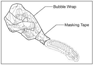
f) While still inside the vehicle, use bubble wrap and masking tape to cover and protect the sensor.
